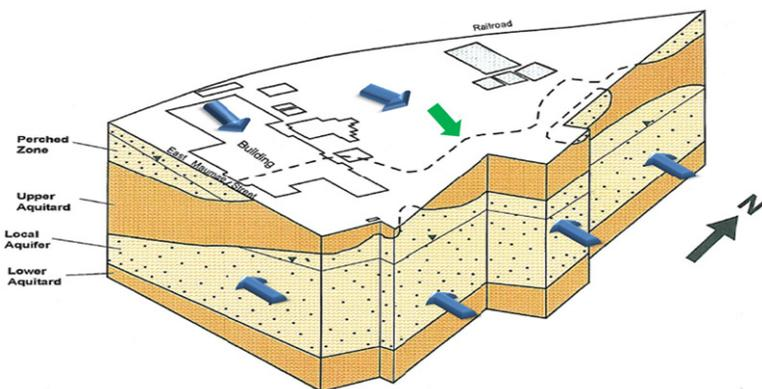
**Figure 1: Basic Hydrogeologic Conceptual Site Model**
