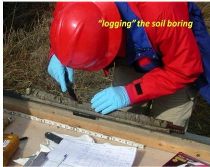
The field geologist inspects the soil core, assessing soil grain size distribution, moisture, odor, staining, and "sniffs" for organic vapors. Note that accurate logging of the subsurface soil is critical when developing the Conceptual Site Model (CSM) and understanding where contamination is currently and where it may go in the future.
